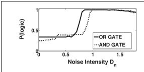
Fig 3. Logic gate performance. OR gate (solid line) and AND gate (dashed line) performances versus the external noise intensity,  $D_n$ .  $\alpha$  and  $\gamma$  values are the same as in the text of [6].
